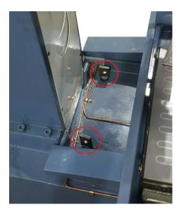
Never lift the machine by its spindle or by cross or magnetic slide wheels. It could damage / bend the sleeve or shaft.
