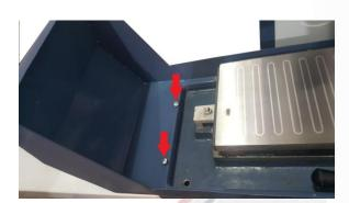
• Lastly push fit the back splash guard first (small one) and then the front splash guard (big one) as shown below.
